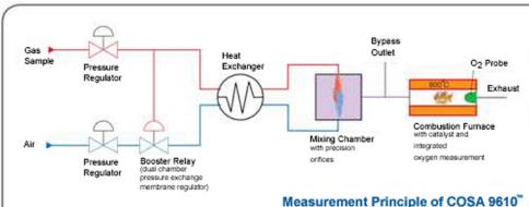
Pressure and temperature of gas sample and instrument air are equalized by means of pre-regulators, a dual chamber pressure exchange membrane regulator (booster relays) and a heat exchanger. The two streams then pass through precision orifices operating at supercritical stage into a mixing chamber. Orifice sizes in the mixing chamber, which are selected based on desired
