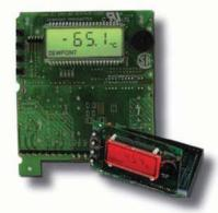
Model XDT-OEM is a stand alone board suitable for mounting in existing enclosures. Connections are made through a pluggable screw terminal block which allows cables to leave the board vertically or horizontally.
