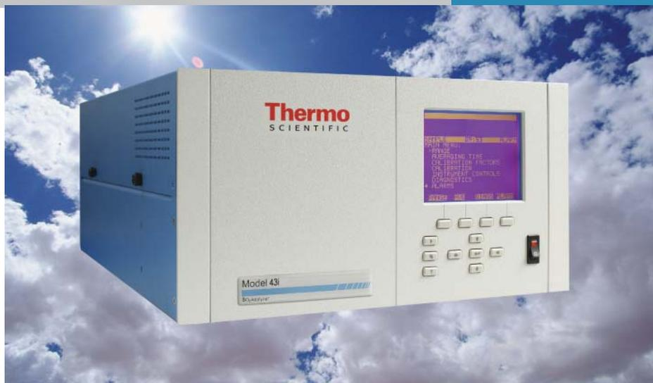
The Thermo Scientific Sulfur Dioxide (SO<sub>2</sub>) Analyzer, Model 43i utilizes pulsed fluorescence technology to measure the amount of sulfur dioxide in the air up to 100 ppm.
