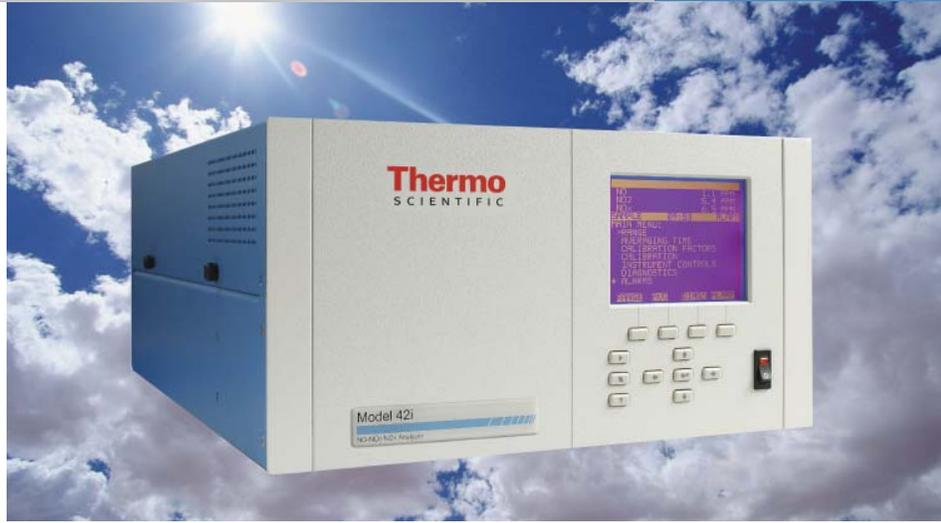
The Thermo Scientific NO-NO<sub>2</sub>-NO<sub>x</sub> analyzer, Model 42i utilizes chemiluminescence technology to measure the amount of nitrogen oxides in the air from sub-ppb levels up to 100ppm.
